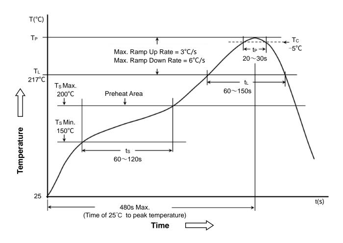
10.2 Classification of peak package body temperature (T<sub>P</sub>) 封装体峰值温度(T<sub>P</sub>)分类
